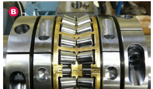
Cooper tapered roller bearing for marine Z-drive propulsion for intermittent thrust loading.
